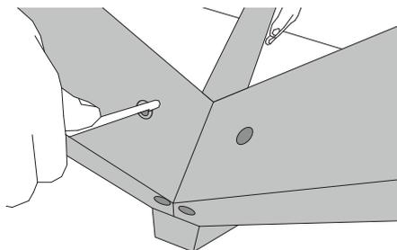
**3.** When all table legs are connected with the frame tighten first all grub screws of the table legs. Afterwards tighten all grub screws of the frame.
