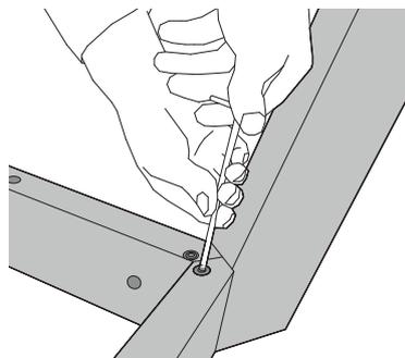
**2.** Put two XS boxes into the top and bottom side of the frame. Stick the table legs onto the frame and fix the connection with the the grub screws (again only slightly!).
