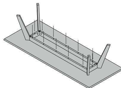
**4.** At last use the cylinder head screws with the disk to fix the frame to the table top.
