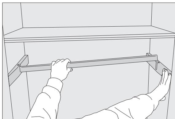
**3.** Now mount the second wooden support for the clothes rail with the shelves supports on the other side of the wardrobe and slide the clothes rail from above into it.
