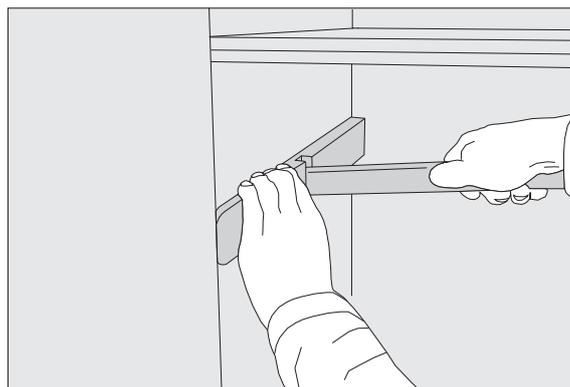
**2.** Slide the clothes rail from above into the wooden support and push it on the side .
