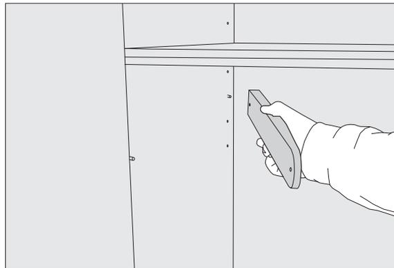
**1.** Mount the wooden support for the clothes rail with the shelves supports on the internal side of the wardrobe.
