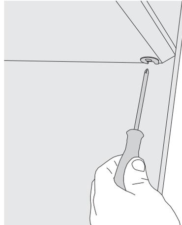
**2.** Afterwards use the cross screw driver to tighten the Rafix connector (just a half turn). Hold the cross screw driver slightly diagonally.
