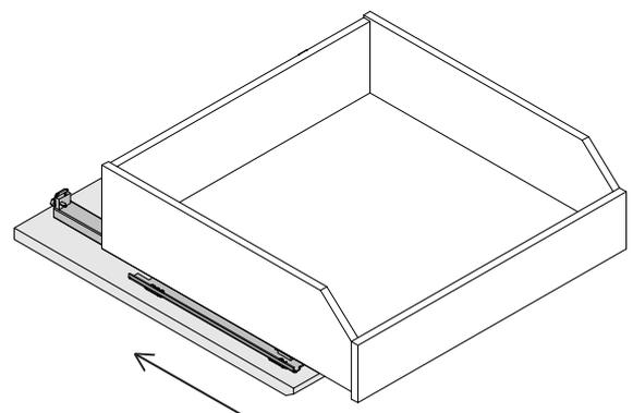
**2.** Pull the fixed runner forwards and put the drawer onto the runner. Now push the drawer back until the runner snaps into the orange box.
