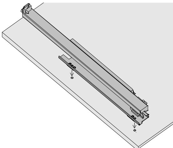
**1.** Screw the runner onto the shelf (already built in). Take care that the runner is at the rearmost position. The side of the shelf with the bigger distance between drilled holes and edge is the one where the door will be placed (the distance is very important for the cup hinges).
