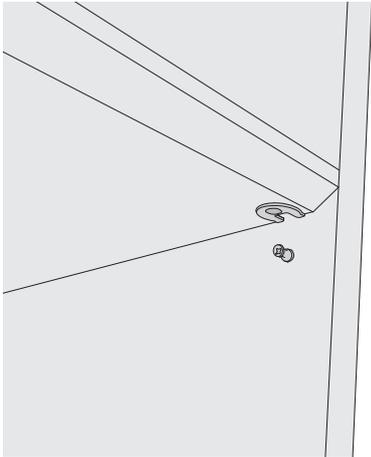
**1.** Screw the metal pin into the side pieces, according to the provided position (as you can see on your individual ZEITRAUM drawing). Press the shelf onto the four metal pins to snap the Rafix- connector.
