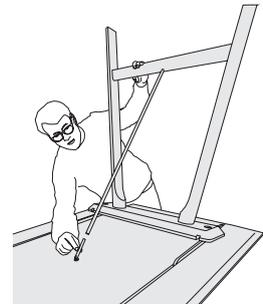
3. Station the trestle with the steel tube onto the orientated hinge peg.
