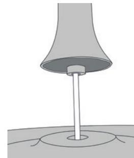
**3.** Insert the tenon into the drilling in the tabletop. Take care the adhesion disc lays flat.
