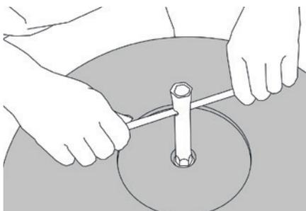
**7.** Tighten the screw nut with the socket wrench **just a little**.
