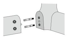
**2.** Assemble pairs of legs and side rails **according to the numbers.** Connect the parts and tighten the connectors with grub srews.
