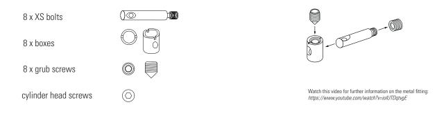
**1.** Screw the XS bolts into the pairs of legs (do not overtighten!) and insert the boxes into the side rails. Align the slots of the boxes with the XS bolts.
