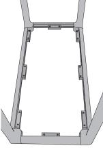
**5.** Place the frame on the bottom side of the tabletop. Slide the mounting blocks into the frame and fix them with pan-head screws.
