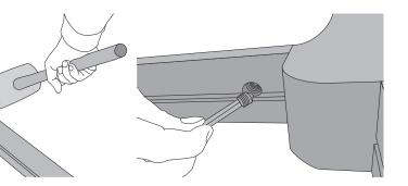
4. Secure the connectors using grub screws. If you cannot tighten the connection, loosen the grub screw and unscrew the bolt by one or two turns. Then connect again.
