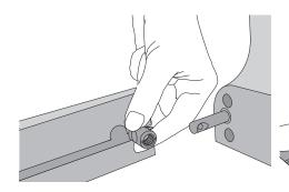
2. Screw the XS bolts into the pairs of legs (do
