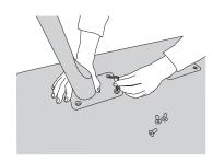
**3.** Stick the four srews in its holes and tighten them up with the allen key.
