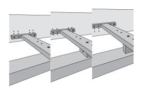
without spacer block: insertion depth 14,5 cm horizontal spacer block: insertion depth 12,5 cm standing spacer block: insertion depth 10,5 cm Use the countersunk screws in the correct length (5x60/80) to fix the spacer block.
