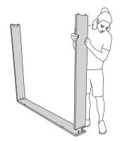
**2.** Attach the head and foot sections and fix them with grub screws.
