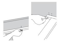
**5.** Fix the side supports using confirmat screws. For mattresses 140 cm or wider, fasten the center rail.
