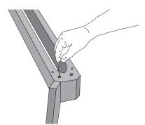
**3.** Tighten the connectors using the allen key. Attach the other legs (1) to the frame (2).
