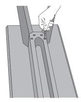
**4.** Place the frame **(2)** on the bench seat **(3)**. Use cylinder head screws to attach the frame.
