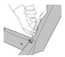
**2.** Put two XS boxes into the top and bottom side of the frame. Stick the table legs onto the frame and fix the connection with the the grub screws (again only slightly!).
