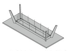
**4.** At last use the cylinder head screws with the disk to fix the frame to the table top.
