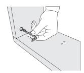
3. Fix the connections with grub screws.
