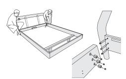
5. Insert the long XS bolts into the headboard (7) and the connector housings into the bed frame. Connect the two parts and fix them using grub screws.
