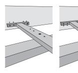
without spacer block: insertion depth 10,5 cm horizontal spacer block: insertion depth 8,5 cm Use the countersunk screws to fix the spacer block.
