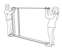
**4.** Attach the second side rail and fix it with grub screws. Also mount the bases (1).
