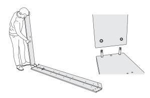
1. Screw the XS bolts into the side rails (4) and insert the connector housings into the footboard (3) and crossbar (2). Connect the two parts. **The footboard needs to be turned correctly:** The drillings in the middle are on the lower edge side.
