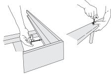
**6.** Attach the support bars **(6)** to the side rail using confirmat screws. If available, mount the center rail **(5)** and middle feet with the countersunk bolts.
