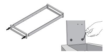
1. Screw XS bolts into foot and head ends and insert the connector housings into the side rails. Align bolts and housings correctly!
