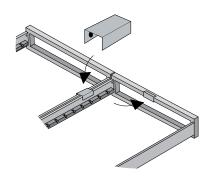
**6.** The GUEST beds can be connected with two aluminium clamps. For this purpose place the beds parallel to each other and join them with the clamps. For non-use please store the clamps upright at the front end of the bed.
