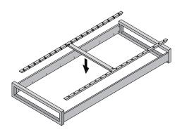
**4.** Fix the mattress frame with confirmat screws. We recommend a 5 cm overhang of the mattress. When two GUEST beds are in use, ensure to use the supports at the same height.
