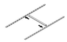
${f 3.}$  Screw XS bolts into the side supports and insert the connector housings into the cross bar. Fit the cross bar between the side supports and tighten the fittings.
