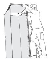
**5.** Screw in the XS bolts in the top of the closet, put in the boxes in the side and place the top, starting on one side, on the closet. After fasten the grub screws.
