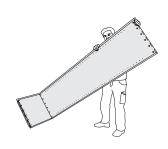
**3.** Place the bottom and Side part upright und put in the back panel in the notch.
