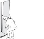
**2.** Place the other side of the closet with the boxes inside on the XS bolts and fasten them with the grub screws.
