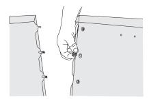
**1.** Screw in the XS bolts in the provided holes in the bottom. Place the boxes in the side of the closet and make sure, the orientation of the box is in the direction of the XS bolts.
