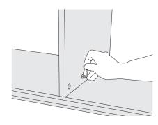
**3.** Place the side pieces onto the XS bolts in the bottom board and fix the side pieces with the grub srews.
