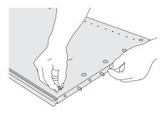
**2.** Put the boxes into the side pieces with the slots of the boxes in direction to the XS bolts (as on the drawing above).
