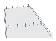
**1.** First mount KIN BASE. Afterwards screw the XS bolts into the holes provided at the bottom board.
