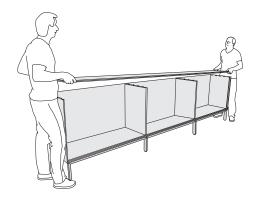
**5.** Screw the XS bolts into the holes provided at the top board. Starting on one side, put the top board onto the sidepieces and fix them with the grub srews.
