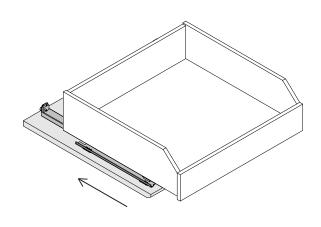
**2.** Pull the fixed runner forwards and put the drawer onto the runner. Now push the drawer back until the runner snaps into the orange box.
