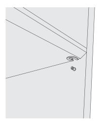
**1.** Screw the metall pin into the side pieces, according to the provided position (as you can see on your individual ZEITRAUM drawing). Press the shelf onto the four metal pins to snap the Rafix- connector.
