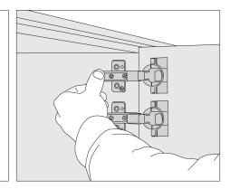
**3.** Hold the door in the open position and hook the hinges onto their mounting plates. Press on the bars to snap them in place against the plates. Now close the door and check the reveal.
