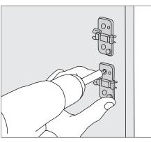
**2.** Attach the mounting plates (remove them from the hinges), the arrow must be facing forwards.
