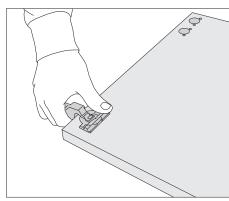
**1.** Press the hinge cups into the holes provided in the doors and turn over the brackets.
