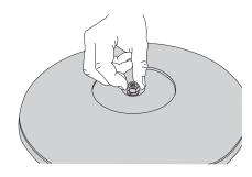
5. ... at last screw in the screw nut.
