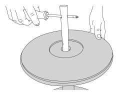
**6.** Tighten the screw nut with the socket wrench.
