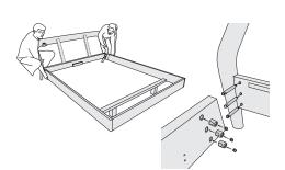
**5.** Insert the long XS dowels into the head-board **(7)** and the connector housings into the bed frame. Connect the two parts and fix them using grub screws.
