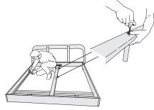
**6.** Attach the support bars **(6)** to the side rails using Confirmat screws. Mount the center rail **(5)** and center support feet **(8)** with the countersunk bolts (M8x50).
