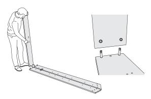
1. Screw the short XS dowels into the side rails (4) and insert the connector housings into the footboard (3) and crossbar (2). Connect the two parts. **The footboard needs to be turned correctly:** The drillings in the middle are on the lower edge side.
