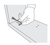
3. Fix the connections with grub screws.
