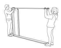
**4.** Attach the second side rail and fix it with grub screws. Mount the bed feet **(1)**.
