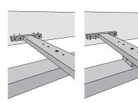
without distance block: insertion depth 10,5 cm horizontal distance block: insertion depth 8,5 cm Use the countersunk screws (5x60) to fix the distance block (8).
