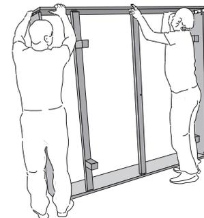
4. Connect the second side rail and fix it with grub screws.
