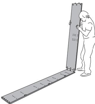
2. Attach the head and footboard to the side rail and fix them with grub screws.
