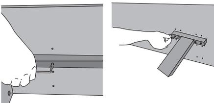
5. Fix the support bars and center rail using Confirmat screws.
