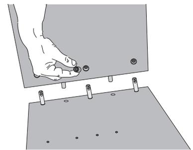
1. Screw the XS dowels into the side rails (2) and insert the connector housings into head and footboard (1). Align dowels and housings correctly!
