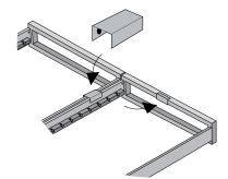
**5.** Insert the rubber caps into the holes in the mattress supports. Fit the sprung slats into the rubber caps.
