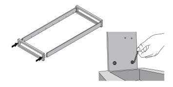
1. Screw XS bolts into foot and head ends and insert the connector housings into the side rails. Align bolts and housings correctly!
