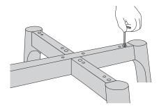
3. Fix all grub screws on the top side of the frame.
