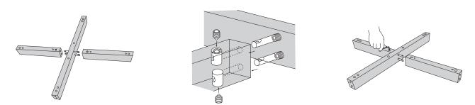
1. Mount the frame cross: screw in the XS steel dowels, insert the connector housings, join the parts and fix the connection with grub screws.
