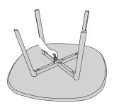
5. ...and mount it with cylinder head screws.
