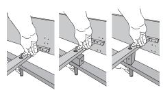
without distance block: insertion depth 16,5 cm horizontal distance block: insertion depth 10,5 cm vertical distance block: insertion depth 6,5 cm
