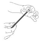
**5.** Screw the sleeve nuts onto the threaded rods (short threaded rods only for lowest position).
