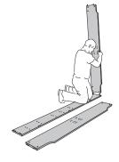
1. Screw XS dowels into side rails (1) and insert the connector housings into the holes. Align dowels and housings correctly! Mount foot and headboard (2) to the side rails.
