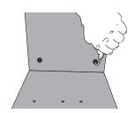
2. Fix the connection with grub screws.
