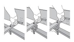
without distance block: insertion depth 16,5 cm horizontal distance block: insertion depth 10,5 cm vertical distance block: insertion depth 6,5 cm
