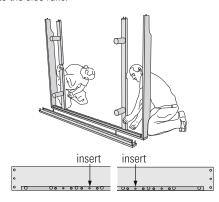
4. Place the bed feet (2) on the crossbars (1) and mount those to the side rail (3). Then attach the second side rail and fix it in place.
