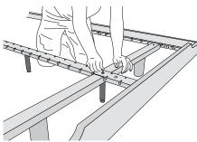
**6.** Mount the adjustable centre feet **(2)** to the centre rail **(5)** using countersunk screws.
