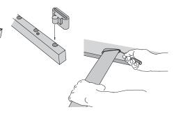
7. Insert the rubber caps into the holes in the mattress supports and fit the sprung slats into the rubber caps.
