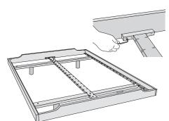
**5.** Place bed on its feet. Insert the centre rail **(5)** and fix it with screws.
