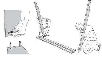
1. Screw XS bolts into side rails (3) and insert connector housings into the foot and head sections (4) and crossbars (1). Align the bolts and housings correctly! Mount foot and headboards to the side rails.
