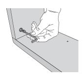
2. Use grub screws to tighten the connections of side rail (3), foot and headboard (4).
