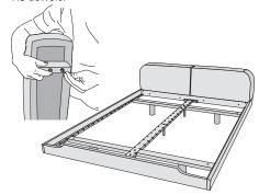
5. Attach the mounting blocks to the bottom of the cushion with the cylinder head screws. Insert the cushions between the head rails (4, 5) the soft side of the cushion facing towards the front.
