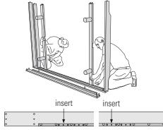
3. Place the two bed feet (2) on the crossbars (1) and attach them to the support bars (6). Then attach the second side rail (3) and fix it in place.
