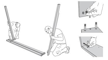
1. Screw XS dowels into side rails (3) and insert the connector housings into the foot and head sections (4) and crossbars (1). Align dowels and housings correctly! Mount foot and headboard (4) as well as the upholstery bar (5) to the side rails and fix with grub screws.
