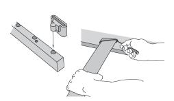
7. Insert the rubber caps into the holes in the mattress supports and fit the sprung slats into the rubber caps.
