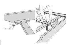
4. Place the bed on its feet. Insert the center rail (6) and fix it with screws. Mount the adjustable center support feet (2) to the center rail (6) using countersunk screws (M8).
