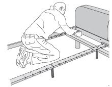
6. Fix the cushions using flat head screws (M6).
