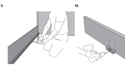
Push the support bars (5) onto the holes in the side rails (4) and secure them with Spax screws.
