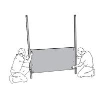
Push the headboard (1) onto the Maxifix bolts of the Reattach the vertical bars. corner posts (6) and tighten the connectors using the allen key.
