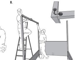
Place the bars of the upper frame (7) in between the corner posts (6) and secure them with frame connectors. Tighten the connectors using an openend wrench.
