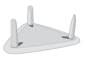
**3.** Place the legs in the milled pocktes on the underside of the tabletop (3).
