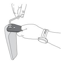
**1.** Screw the mounting plates **(2)** onto the legs **(1)** using countersunk bolts (M10).
