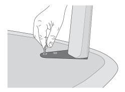
4. Fix the mounting plates with screws.
