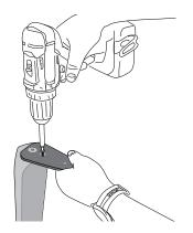
**2.** Secure the mounting plates by screwing the Spax screw into the provided holes.
