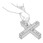
2. Fix the connection with grub screws.
