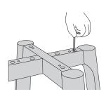
**7.** Fix all grub screws on the top side of the frame.
