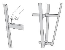
**6.** Mount the lower cross to the leg. Afterwards, mount the remaining legs. Assembly is easier when the table is upside down.
