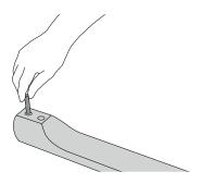
**3.** Screw in the XS steel dowels (M8) into the legs.
