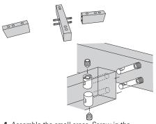
**1.** Assemble the small cross. Screw in the XS steel dowels (M6), insert the connector housings and connect the parts.
