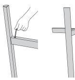
**6.** Mount the cross to the leg. Afterwards, mount the remaining legs. Assembly is easier when the table is upside down.
