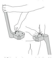
**4.** Tighten the grub screws on both sides of the block.
