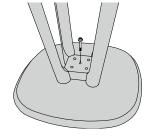
**8.** Insert the cylinder head screw with the flat washer.
