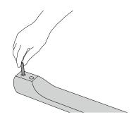
1. Screw in the XS steel dowels (M8).
