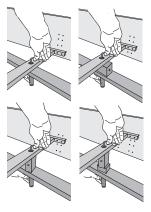
without distance block: insertion depth 24,5 cm horizontal big distance block: insertion depth 18,5 cm vertical big distance block: insertion depth 14,5 cm both distance blocks: insertion depth 10,5 cm
