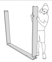
**2.** Attach the head and foot sections to the side rail and fix them with grub screws.
