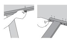
**5.** Fix the side supports using confirmat screws. For mattresses 140 cm or wider, fasten the center rail.
