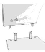
**1.** Screw the bolts into the side rails and insert the connector housing into the head and foot sections. Align bolts and housing correctly!
