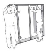
4. Connect the second side rail and fix it with grub screws.
