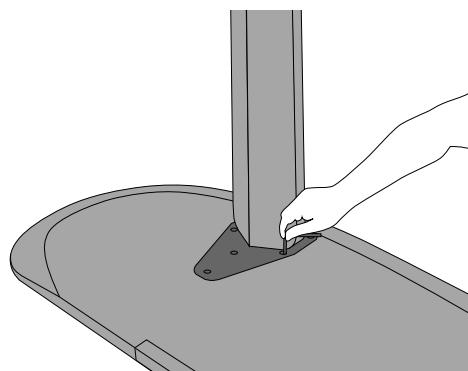
2. Place the tabletop upside down and position the leg. Screw the mounting plate to the tabletop using countersunk screws M6.
