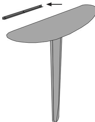
3. Mount the mounting angle to the wall. Use appropriate wall plugs and screws depending on the wall condition.
