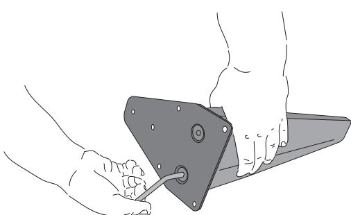
1. Screw the mounting plate to the leg using countersunk screws M10.
