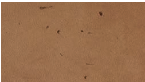
Fork stitches , can vary in depth, so that usually only covered leathers can be made from these hides.
