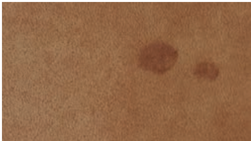
Small rot and insect bites , these dark spots on the hide are not dark spots in terms of quality.
