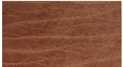
Mast wrinkles , occur in the neck area of the hide and give the leather a pithy, rustic appearance appreciated by connoisseurs.
