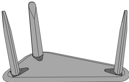
2. Place the legs in the milled pocktes on the underside of the tabletop.
