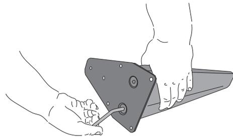
1. Screw the mounting plates on the legs using countersunk screws M10.
