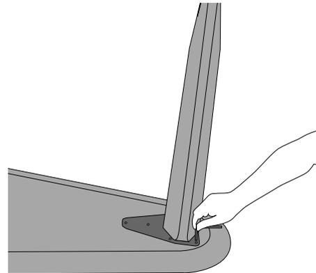
3. Fix the mounting plates with countersunk screws M6.
