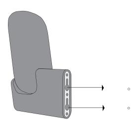
${\bf 2.}$  Place the hook with the keyhole fittings on the screw heads. If necessary, adjust the screws.
