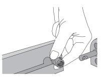
**2.** Screw the long XS steel dowels into the legs (do not overtighten!) and insert the connector housings into the frame rails. Screw the short XS steel dowels into the center of the frames rails and reinforcing cross and fit the housings to the reinforcing cross. When aligning the housings, ensure that the slots point towards the intersecting holes.
