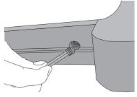
**4.** Secure the connectors using grub screws. If you cannot tighten the connection, loosen the grub screw and unscrew the steel dowel by one or two turns. Then connect again.
