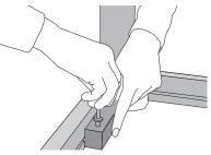
**6.** Place the frame on the bottom side of the tabletop. Slide the mounting blocks into the frame and fix them with flat head screws.
