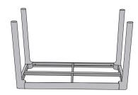
**5.** Next, assemble the reinforcing cross. Mount the long frame rails on the reinforcing cross and fix them in place, then place the short frame rails with the legs on the sides and mount them.
